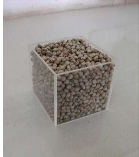
Plate 4.6 Measurement of bulk density of pigeon pea grains.
