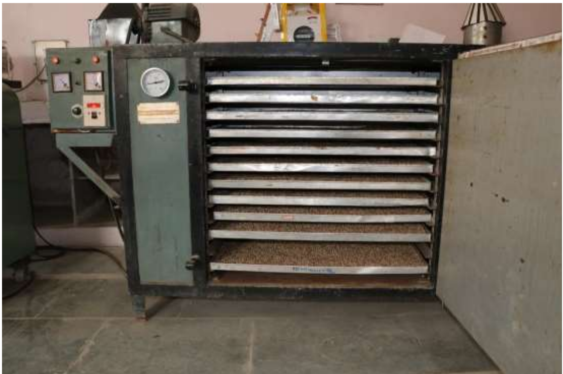
Drying of enzyme treated pigeon pea grains in the tray dryer
