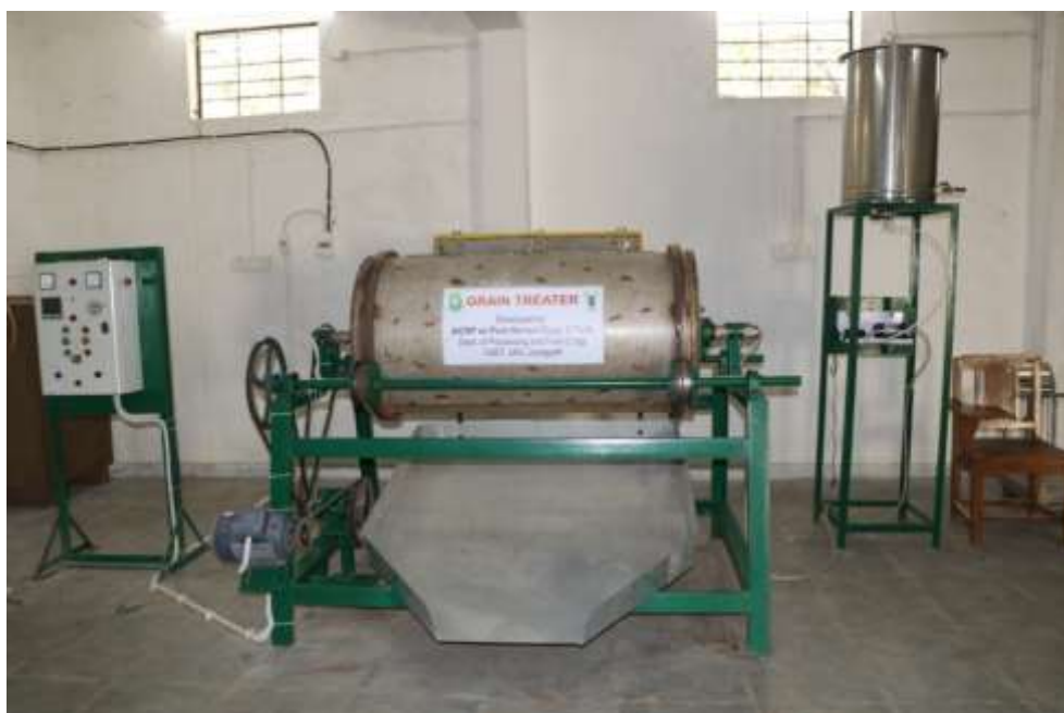
Plate 4.12 Grain treater used for giving enzymatic pre-treatment to pigeon pea grains.
