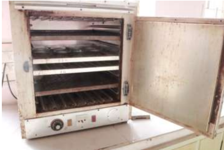
Plate 4.3 Moisture content determination of pigeon pea grains using hot air oven.
