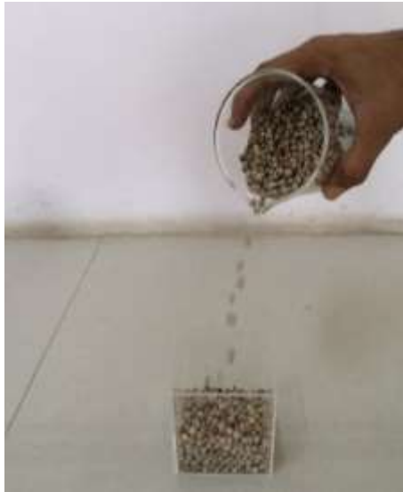
Plate 4.6 Measurement of bulk density of pigeon pea grains.
