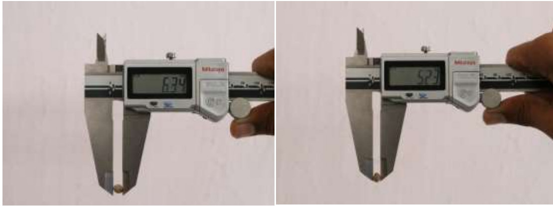
Plate 4.4 Measurement of physical dimensions of pigeon pea grains using vernier caliper.
