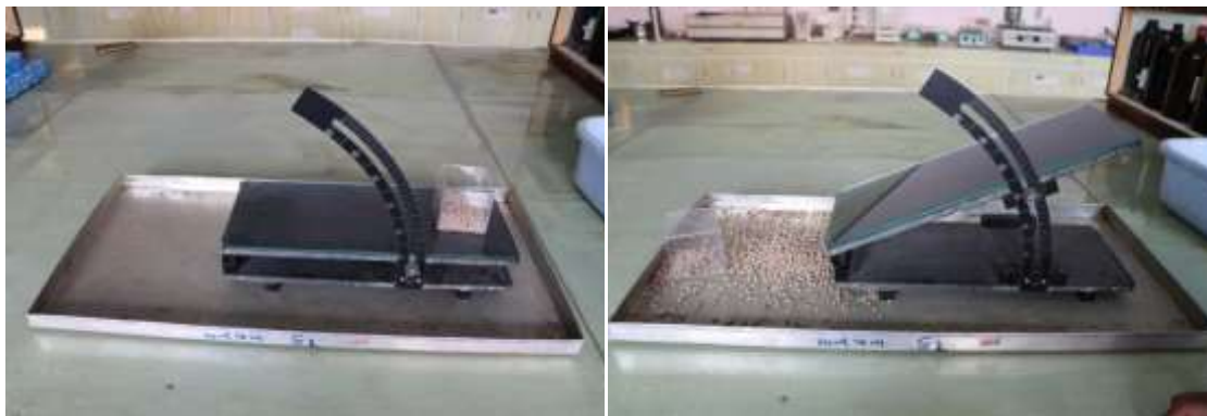
Plate 4.9 Measurement of coefficient of friction of pigeon pea grains
